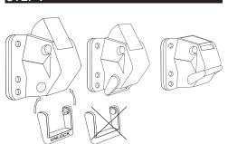
Install red unlocking bar in hole on one side with unlock letters up. Then straddle the housing and pop in the opposite side.
